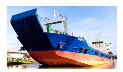
1450.030 TONNES LOA, Length Overall 78.00 Meters Light Ship
